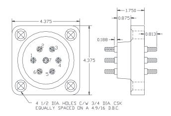
7 Brass Feed Through Studs Clamping Supplied with Hardware 1/4 Brass Nuts Brass Washers Buna "O" Ring Metric Configuration Available
