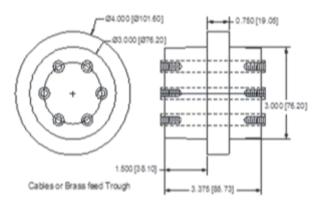
7 Brass Studs Feed Through Also produced with Cables TEW or Tefzel Any Length regired
