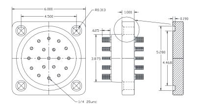
19 Brass Feed Through Supplied with Hardware 1/4 Brass Nuts Brass Washers Buna "O" Ring Metric Configuration Available
