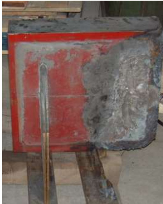
What we received from the customer (it was a 4 bus bars LV Bushing)
