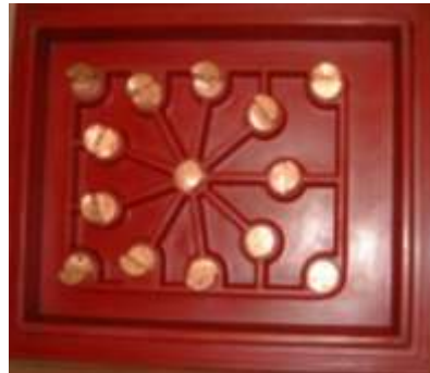
69 KV Selector Board for LTC
