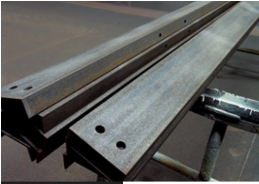
Left: Pieces of metal that has recently been grit blasted in the company's new facility. Right: the company boasts a wide range of fabricating processes, including a CNC cutting table.
