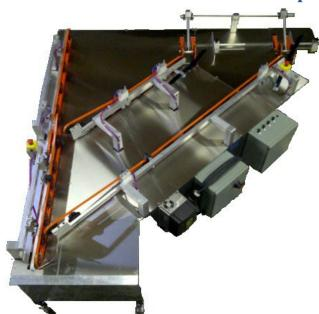
The Econo 3 Deserter can separate up to three nested half-fold impressions, running up to 75,000 impressions per hour. The maximum production yield is 180,000 IPH. The Econo 3 Deserter can also be used to separate two products, or simply the web stream can pass directly through the Econo 3 Deserter unaltered, thereby reducing the need to move the unit.
